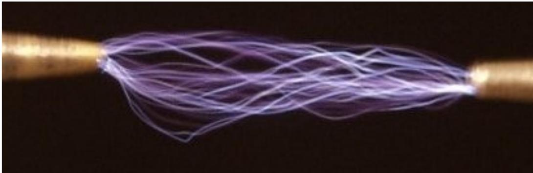
In this image a Tesla coil spark is filmed with a  $\frac{1}{2}$  second exposure to actually capture many discharges
