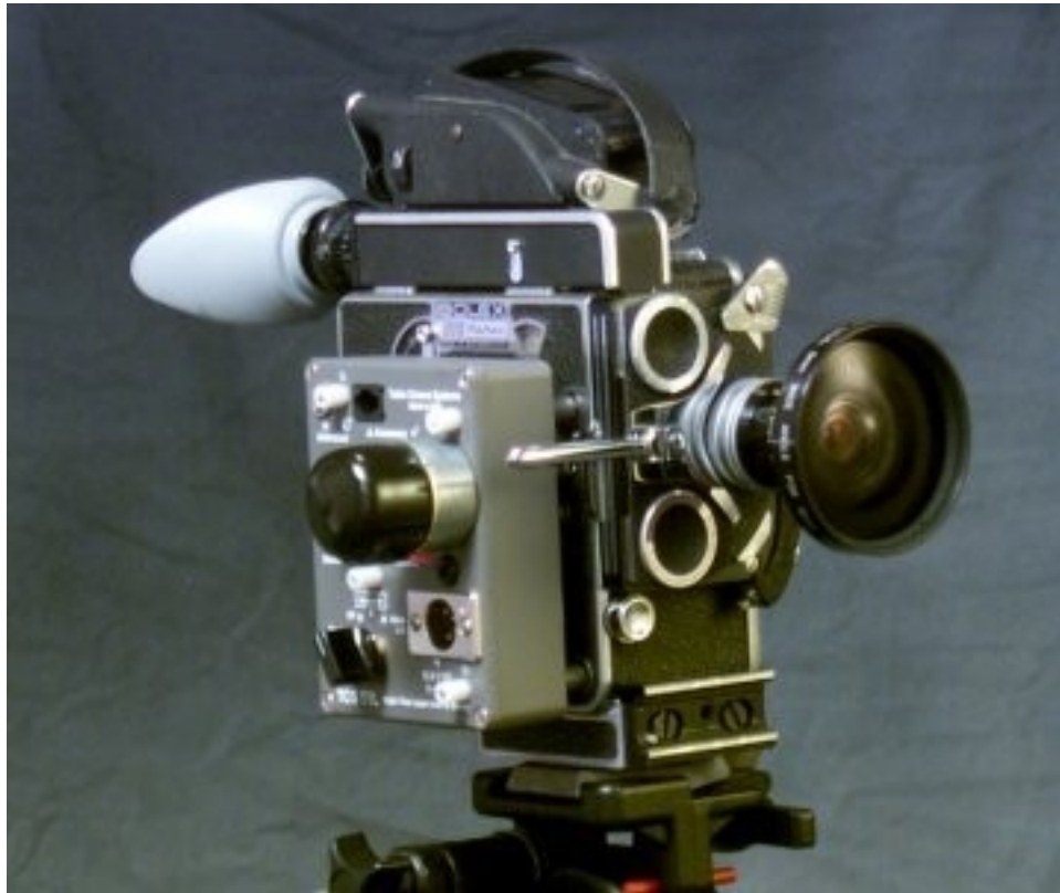
Bolex 16 mm camera with a Tobin time-lapse motor runs on 12 volts DC
